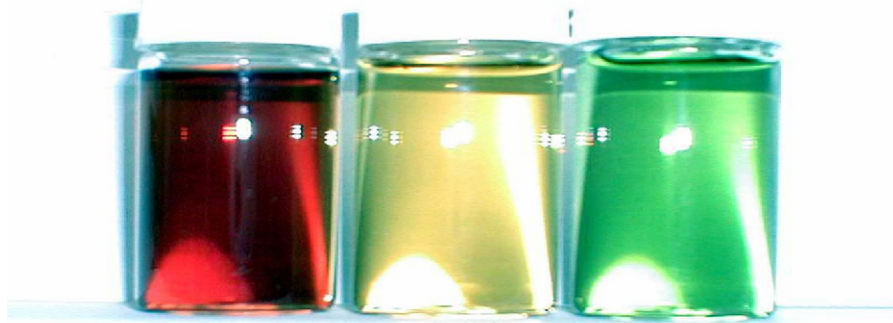
Fig. 4. SSW colour during test conducted with \text{Cu}(\text{NO}_3)_2 in absence of oxygen. (samples left to right: (1) SSW at beginning of test, (2) SSW immediately after completion of test, (3) SSW after exposure to air for \sim 1 h).
