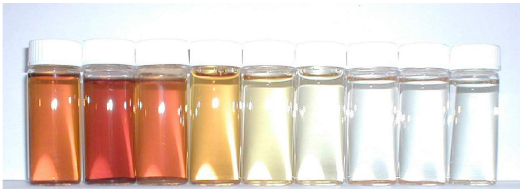
Fig. 9. Colour change during WPO of SSW. Samples from left to right- 0, 5, 10, 18, 28, 43, 60, 75, 90 min). Conditions: pH_i = 3.5 , total H_2O_2 added = 51 g/L (6 equal additions at 0,7,12, 20, 30 and 45 min), t = 90 min, T = 150^\circ C .
